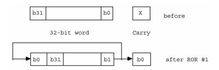
After n of these rotates, the old bit n is in the bit 0 position; the old bit (n-1) is in bit 31 and in the carry flag.
