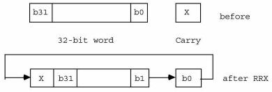
The old bit 0 is shifted into the carry. The old content of the carry is shifted into bit 31.
